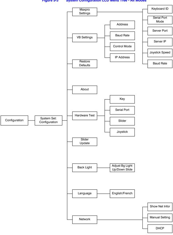
Figure 5-3 System Configuration LCD Menu Tree - All Modes
